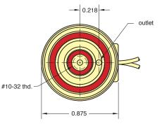
threaded, 7/32" deep mounting holes. Manifold models are equipped with a bottom stud, 5/32" long with #10-32 thread, which fits Clippard standard and special manifolds, accessory valves and subplates. Spanner holes in the valve body permit tightening.
